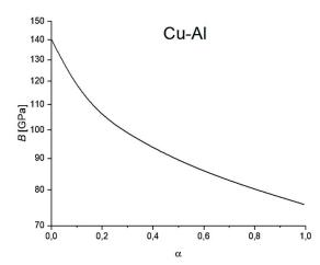
Fig. 2. Dependence of the bulk modulus of Cu-Al on the percentage composition.
