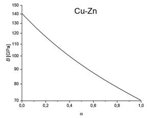
Fig.1. Dependence of the bulk modulus of Cu-Zn on the percentage composition.
