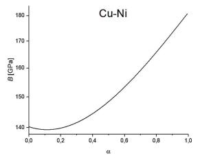
Fig. 3. Dependence of the bulk modulus of Cu-Ni on the percentage composition.
