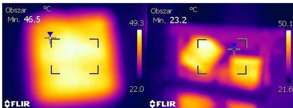
Fig. 9 Thermograms of the samples after compressive (left) and tensile strength (right) tests performed in temperature 50°C
