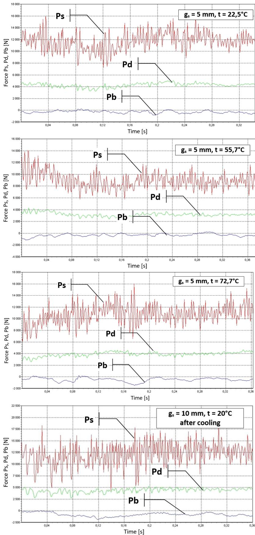
**Fig. 6** The courses of  $P_s$ ,  $P_d$  and  $P_b$  force values for cuts with a depth of 5 mm at temperatures 22.5°, 55° and 72°C and a cut with a depth of 10 mm for temperature 20°C after sample cooling
