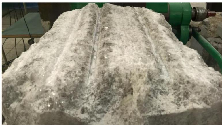
**Fig. 5 View of the sample with the cuts (depths in turn from the left  $g_s$  5, 10 and 7 mm) made at a temperature of about 20°C, after cooling the sample**
