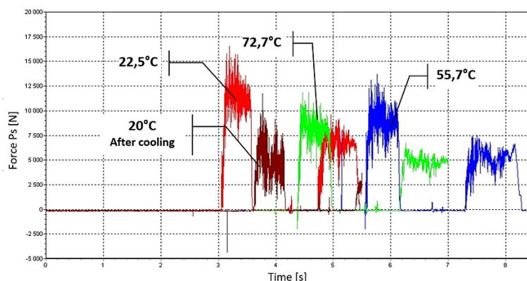
**Fig. 7  $P_s$  force value for cutting depth 5 mm for three different sample temperature and after sample cooling**
