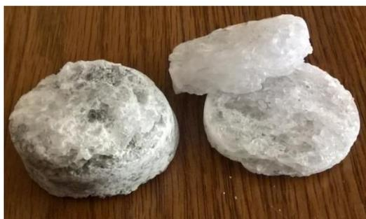
Fig. 1 View of destroyed sample after drilling using a Trepaner drill
