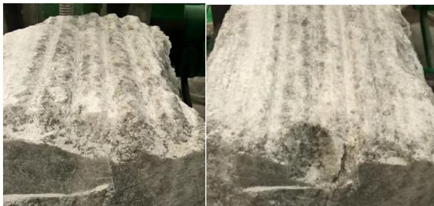
**Fig. 3 View of obtained cuts for cutting depth of 5 mm, with temperature about 22°C (left) and about 80°C (right)**
