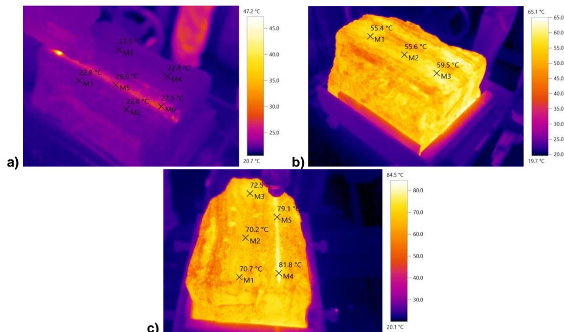
**Fig. 4 Thermograms of a sample surface and performed cut during cutting with temperature: a) 22,5°C, b) 57°C and c) 72°C**
