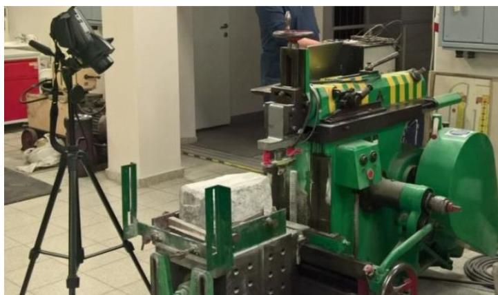
Fig. 2 View of special laboratory test stand for cutting resistance tests with a strain-gauge head
