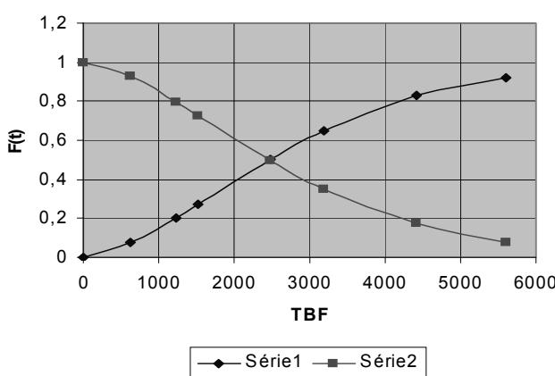
Fig. 5 Reliability and distribution function-TBF
