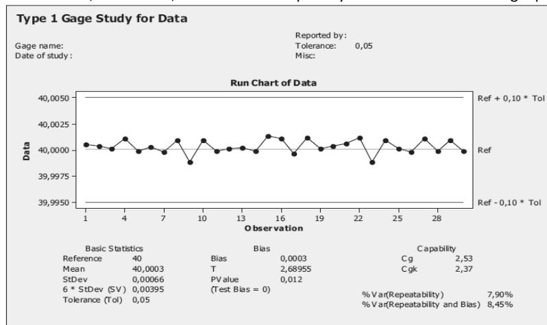
**Fig. 3 Behaviour of the measured values deviation**
