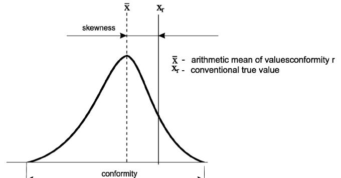
Fig. 1 Skewness and conformity of measurement
